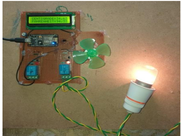
Fig.8. Images of accurate room temperature controller using ESP8266
